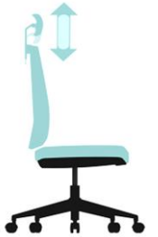
Neck-rest height adjustment
